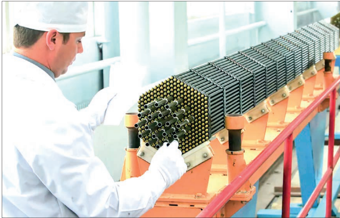
Nuclear power reactor fuel assembly at the Novosibirsk Chemical Concentrate Works. PHOTO: PIX FOR VISUAL PURPOSE/ SPUTNIK
