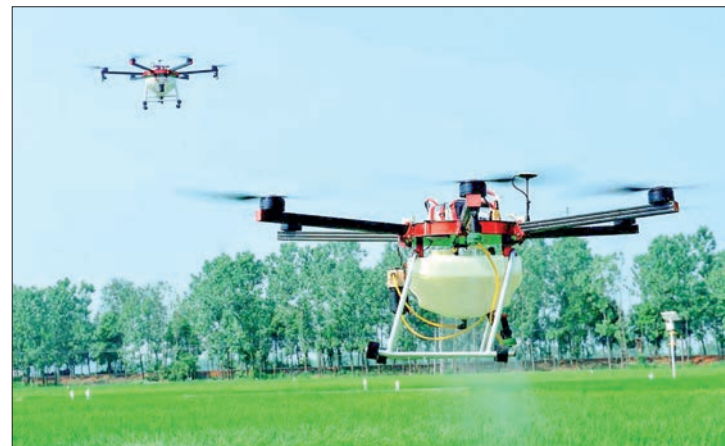
Agricultural drones are unmanned aerial vehicles (UAVs) that are increasingly being utilized in modern farming practices. One specific application of agricultural drones is the spraying of pesticides on crops. PHOTO: PIX FOR VISUAL PURPOSE/AFP
