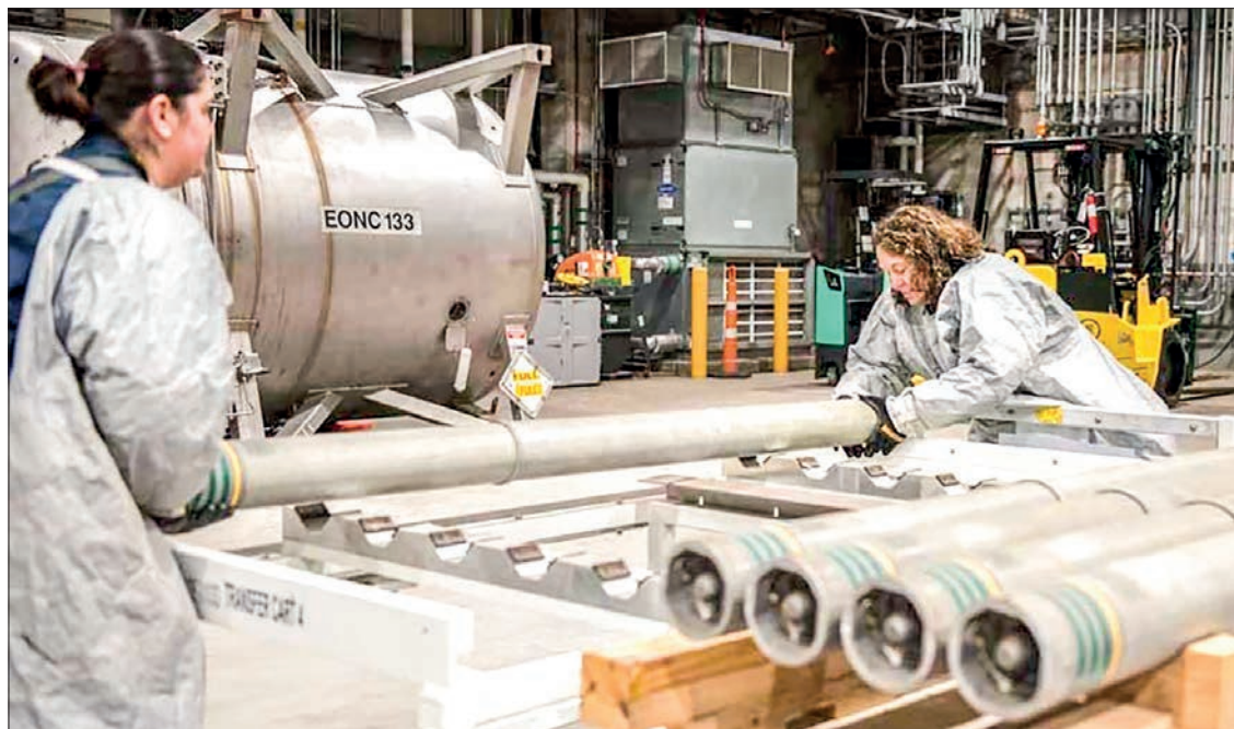
Operators move M55 rockets containing VX nerve agent from a pallet to a transfer cart to begin the destruction process at the Blue Grass Chemical Agent-Destruction Pilot Plant 15 April 2022. PHOTO: PIX FOR VISUAL PURPOSE/US ARMY/FILE
